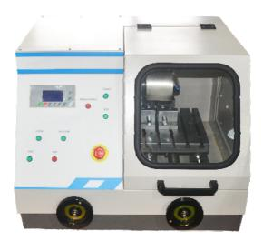
Model iCut-857/858 cutting machine is composed of main machine, electric control box, cutting room, motor, cooling system, cutting grinding wheel and other parts.
